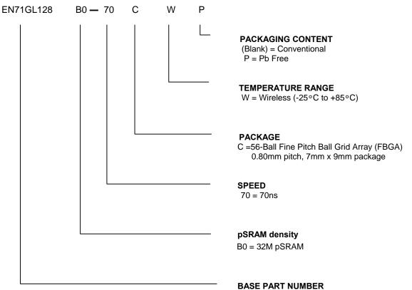
EN = Eon Silicon Solution Inc. 71GL = Multi-chip Product (MCP)
