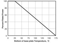
Derating (thermal resistance): 0.666W/°K (1.5K/W). Without a heatsink, when in free air at 25°C, the TEH100 is rated for 3.5W. Derating for temp. above 25°C is 0.0234W/°K
