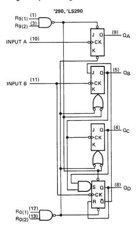
NOTES: A. Output  $\Omega_A$  is connected to input B for BCD count.
