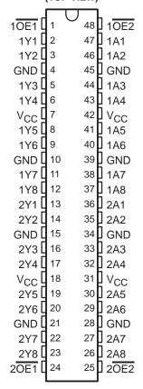
To ensure the high-impedance state during power up or power down,  $\overline{OE}$  should be tied to  $V_{CC}$  through a pullup resistor; the minimum value of the resistor is determined by the current-sinking capability of the driver.
