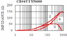
FREQUENCY (MHz) RDC: 0.10 Ω Rated current:500 mA
