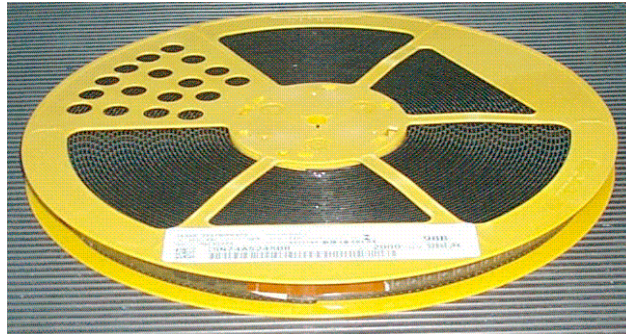
Figure 15. Loaded Reel (Not Moisture Sensitive)
