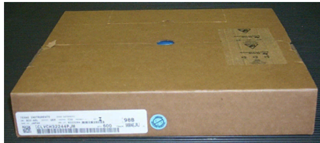
Figure 18. Dry-Packed Tape-and-Reel Configuration
