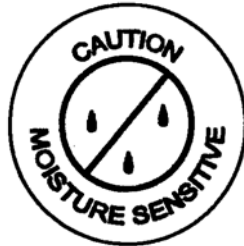
Figure 19. Moisture-Sensitive Identification (MSID) Label
