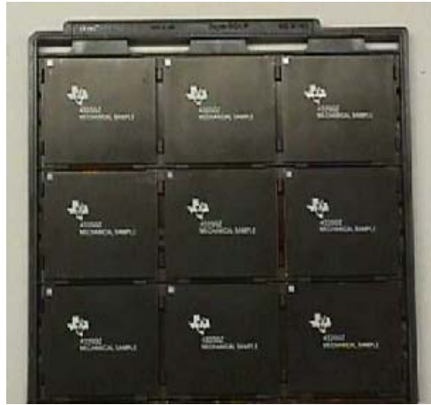
Figure 6. JEDEC Tray With Properly Arranged Units
