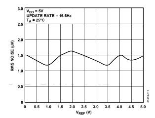
Figure 9. AD7788/AD7789 Noise vs. VREF
