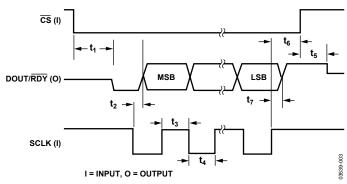
Figure 3. Read Cycle Timing Diagram
