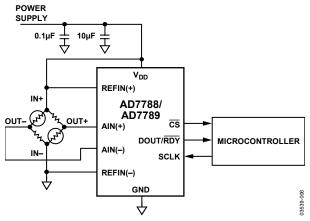
Figure 10. Basic Connection Diagram
