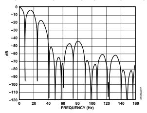
Figure 6. Frequency Response with 16.6 Hz Update Rate
