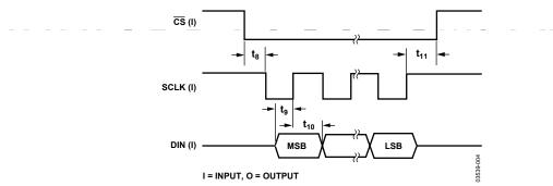
Figure 4. Write Cycle Timing Diagram
