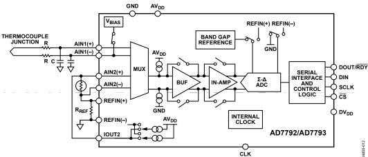
Figure 20. Thermocouple Measurement Using the AD7792/AD7793
