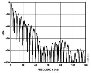
Figure 13. Filter Profile with Update Rate = 4.17 Hz
