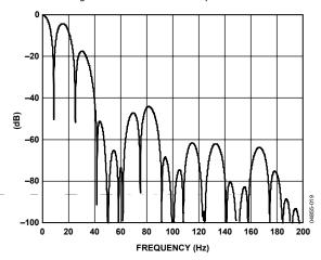
Figure 14. Filter Profile with Update Rate = 16.7 Hz
