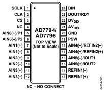
Figure 5. Pin Configuration
