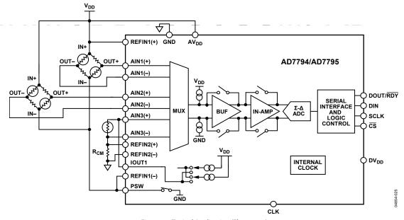
Figure 24. Typical Application (Flowmeter)
