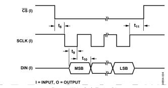
Figure 4. Write Cycle Timing Diagram
