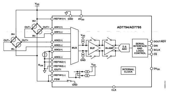
Figure 12. Basic Connection Diagram
