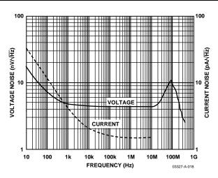
Figure 19. Voltage and Current Noise vs. Frequency
