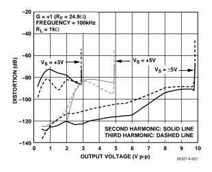
Figure 22. Harmonic Distortion vs. Output Amplitude
