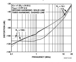
Figure 24. Harmonic Distortion vs. Frequency and Load
