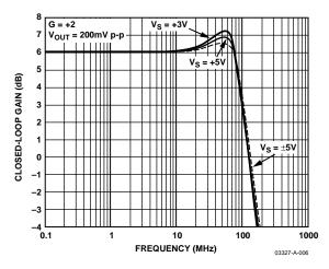
Figure 7. Small Signal Frequency Response for Various Supplies
