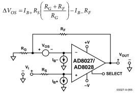
Figure 56. Op Amp DC Error Sources
