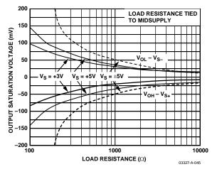
Figure 46. Output Saturation Voltage vs. Output Load
