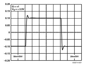
Figure 28. Small Signal Transient Response
