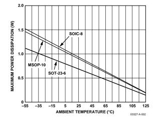
Figure 3. Maximum Power Dissipation vs. Ambient Temperature
