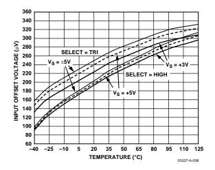
Figure 39. Input Offset Voltage vs. Temperature
