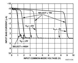
Figure 37. Input Bias Current vs. Input Common-Mode Voltage
