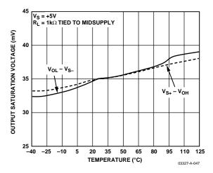
Figure 48. Output Saturation Voltage vs. Temperature
