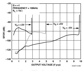
Figure 2. SFDR vs. Output Amplitude
