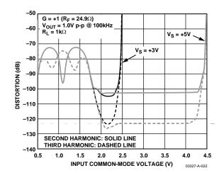
Figure 23. Harmonic Distortion vs. Input Common-Mode Voltage, SELECT = High
