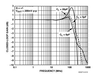
Figure 13. AD8028 Small Signal Frequency Response for Various CLOAD
