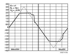
Figure 33. Input Overdrive Recovery
