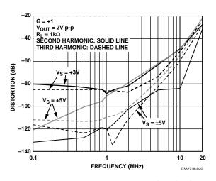
Figure 21. Harmonic Distortion vs. Frequency and Supply Voltage
