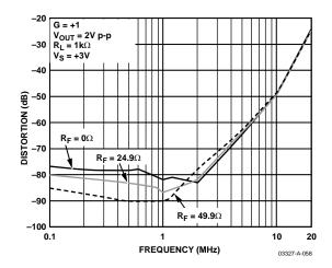
Figure 59. SFDR vs. Frequency and Various R<sub>F</sub>
