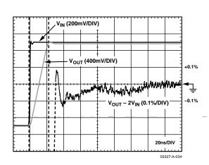
Figure 35. 0.1% Short-Term Settling Time
