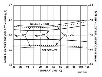
Figure 36. Input Bias Current vs. Temperature
