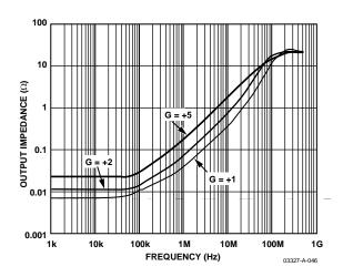
Figure 47. Output Enabled— Impedance vs. Frequency
