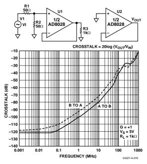
Figure 17. AD8028 Crosstalk Output to Output
