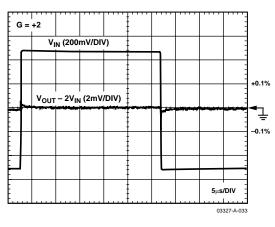
Figure 34. Long-Term Settling Time
