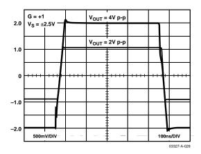
Figure 29. Large Signal Transient Response, G = +1
