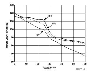
Figure 49. Open-Loop Gain vs. Load Current
