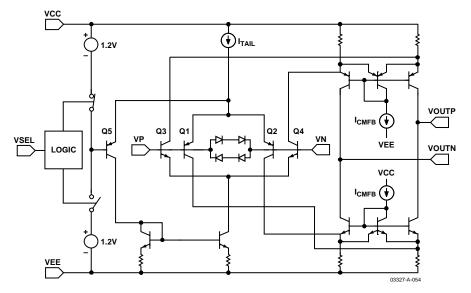
Figure 55. Simplified Input Stage
