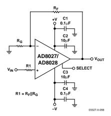
Figure 57. Wideband Noninverting Gain Configuration
