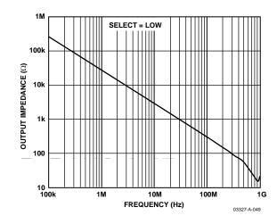
Figure 50. Output Disabled—Impedance vs. Frequency
