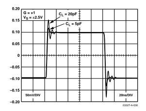
Figure 31. Small Signal Transient Response with Capacitive Load
