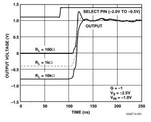
Figure 52. Enable Turn-On Timing
