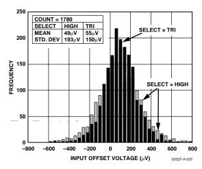
Figure 38. Input Offset Voltage Distribution
