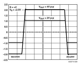
Figure 30. Large Signal Transient Response, G = +2
