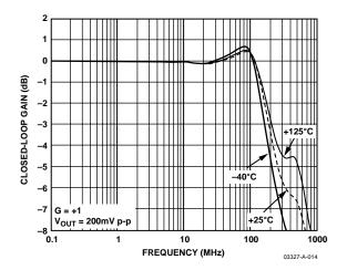
Figure 15. AD8028 Small Signal Frequency Response vs. Temperature
