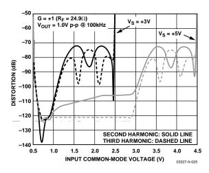
Figure 26. Harmonic Distortion vs. Input Common-Mode Voltage, SELECT = Three-State or Open
