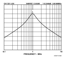
Figure 63. Band-Pass Filter Response
