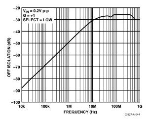
Figure 45. Off Isolation vs. Frequency
