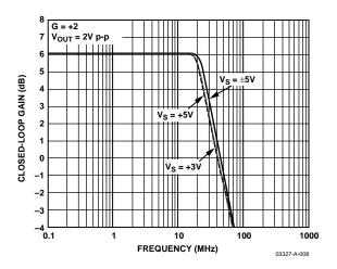
Figure 9. Large Signal Frequency Response for Various Supplies
