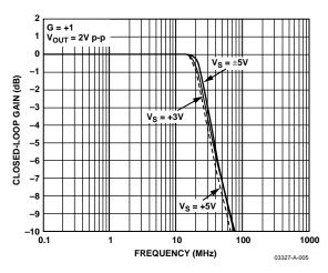
Figure 6. Large Signal Frequency Response for Various Supplies
