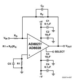
Figure 58. Wideband Inverting Gain Configuration
