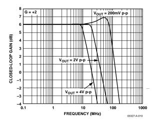
Figure 11. Frequency Response for Various Output Amplitudes
