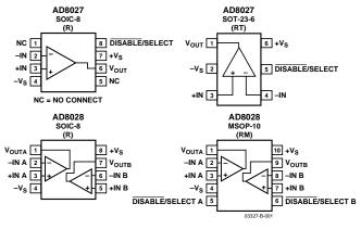
Figure 1. Connection Diagrams (Top View)
