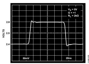
Figure 35. AD8051/AD8052 200 mV Step Response;  $V_S = 5 V$ , G = +1
