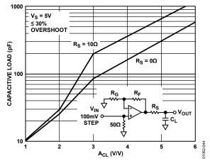
Figure 45. AD8054 Capacitive Load Drive vs. Closed-Loop Gain
