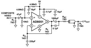
Figure 52. Single-Supply Composite Video Line Driver
