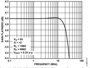
Figure 13. AD8051/AD8052 0.1 dB Gain Flatness vs. Frequency; G = +2
