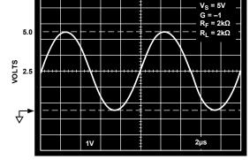
Figure 37. Output Swing; G = -1,  $R_L = 2 k\Omega$
