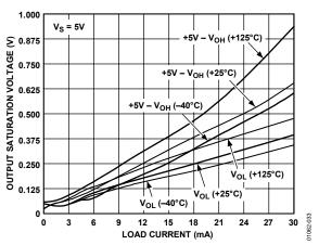
Figure 33. AD8054 Output Saturation Voltage vs. Load Current
