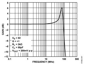
Figure 42. AD8051/AD8052 Closed-Loop Frequency Response;  $C_L = 50 \, pF$
