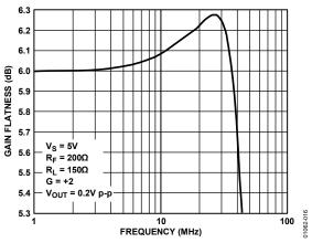
Figure 16. AD8054 0.1 dB Gain Flatness vs. Frequency; G = +2
