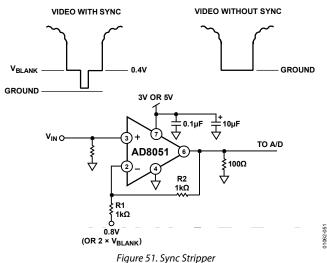
The video signal plus sync is applied to the noninverting input with the proper termination. The amplifier gain is set to 2 via the two 1 k $\Omega$  resistors in the feedback circuit. A bias voltage must be applied to R1 so that the input signal has the sync pulses stripped at the proper level.
