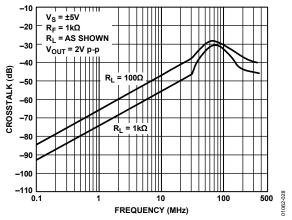
Figure 28. AD8054 Crosstalk (Output-to-Output) vs. Frequency
