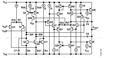
Figure 40. AD8051/AD8052 Simplified Schematic
