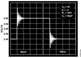
Figure 43. AD8051/AD8052 200 mV Step Response;  $C_L = 50 \text{ pF}$
