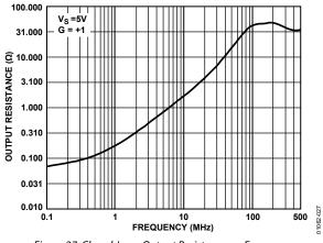
Figure 27. Closed-Loop Output Resistance vs. Frequency
