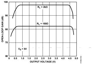
Figure 32. Open-Loop Gain vs. Output Voltage
