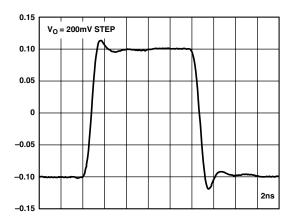
TPC 23. AD8074 Small Signal Pulse Response (R<sub>L</sub> = 1 k $\Omega$ , C<sub>L</sub> = 5 pF)
