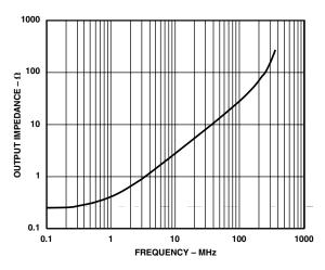
TPC 18. AD8074 Output Impedance vs. Frequency; Enabled
