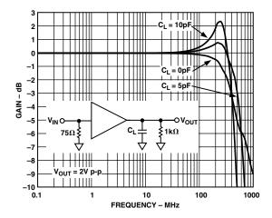
TPC 3. AD8074 Frequency Response vs. Capacitive Load
