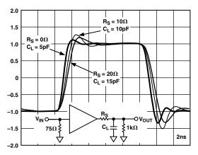
Figure 2. Driving Capacitive Loads
