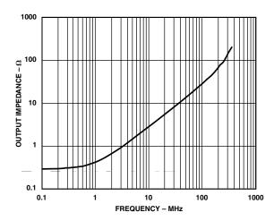
TPC 21. AD8075 Output Impedance vs. Frequency; Enabled
