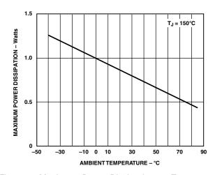
Figure 1. Maximum Power Dissipation vs. Temperature
