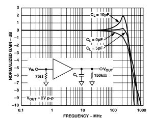
TPC 6. AD8075 Frequency Response vs. Capacitive Load
