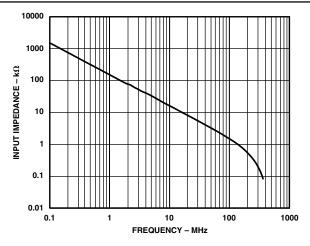
TPC 20. AD8075 Input Impedance vs. Frequency
