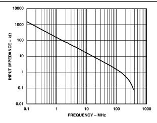
TPC 17. AD8074 Input Impedance vs. Frequency
