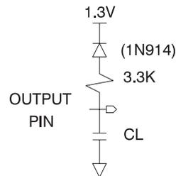
Note:  $C_L = 100 \text{ pF}$  including jig capacitance, except for the -45 devices, where  $C_L = 30 \text{ pF}$ .
