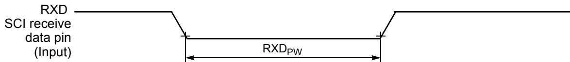
Figure 10-16 RXD Pulse Width
