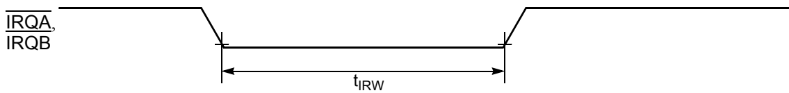
Figure 10-6 External Interrupt Timing (Negative Edge-Sensitive)
