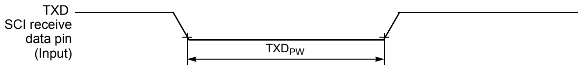
Figure 10-17 TXD Pulse Width
