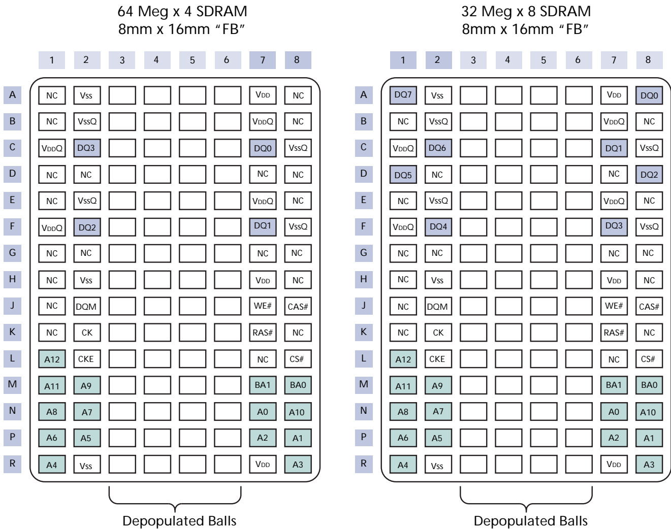
Figure 5: 60-Ball FBGA Assignment (Top View)
