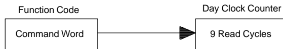
SEQUENCE: PROGRAM MODE, READING THE 9-BIT NUMBER OF DAYS COUNTER Figure 6B
