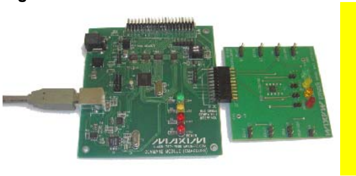
Figure 1. CMAXQUSB with DS28CZ04 EV board
