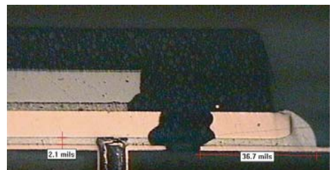
81% paste coverage, encroached via, 2.1 mil standoff
