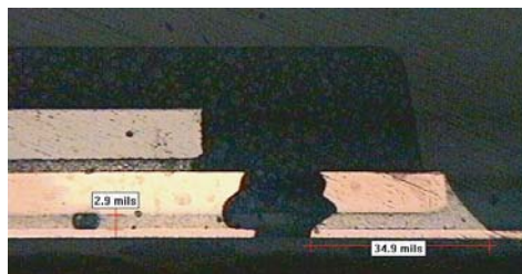
50% paste coverage, plugged via, 2.9 mil standoff
