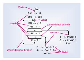
Note the example of algorithm in AB contains only one label name: "Sub", and the "MO", "M1", and "M2" names are absent. In the classical assembler the branch addressing is carried out by labels' names. The use on multiple branch and label names result in a listing crammed with vast number of labels names which are inevitable ballast.
