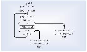
The above subroutine example will be looked in the following way in AB: Five base elements are used in Algorithm Builder for the building of program construction. There are:
