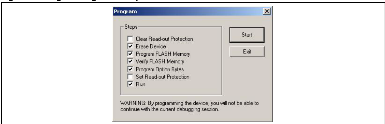
Figure 10. Programming the Microprocessor
