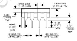
\*DIMENSIONS DO NOT INCLUDE MOLD FLASH OR PROTUSIONS. MOLD FLASH OR PROTUSIONS SHALL NOT EXCEED  $0.010^\circ\ (0.254\mathrm{mm})$
