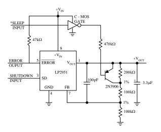
**Open Circuit Detector for 4 to 20mA Current Loop**
