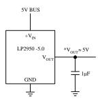
\*Minimum Input-Output voltage ranges from 40mV to 400mV, depending on load current. Current limit is typically 160 mA
