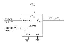
\*Minimum Input-Output voltage ranges from 40mV to 400mV, depending on load current. Current limit is typically 160 mA
