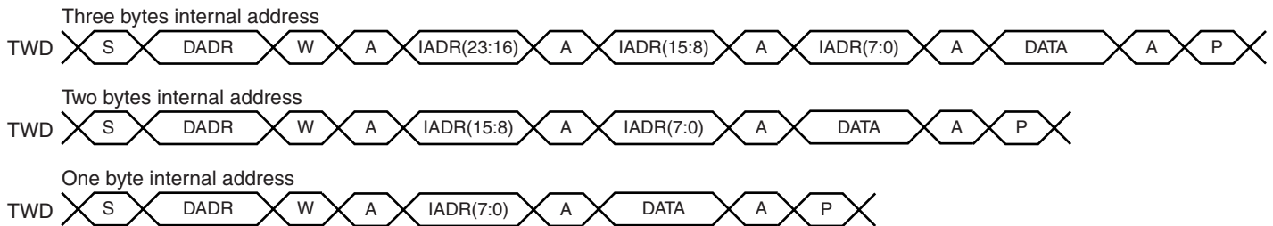
Figure 29-11. Master Write with One, Two or Three Bytes Internal Address and One Data Byte
