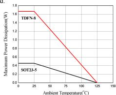
**Figure 5. Power Dissipation for EUP7907 Packages**The EUP7907 is available in two standard packages: TDFN-8 and SOT23-5 packages.
