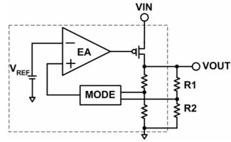
Figure 4. Output Voltage Select Circuit
