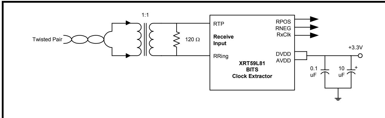
FIGURE 12. CEPT APPLICATION FOR COAXIAL INTERFACE
