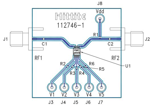
\* R2 - R6= 100 Ohm. These resistors are optional and may be used to enhance decoupling of the RF path from the control inputs.
