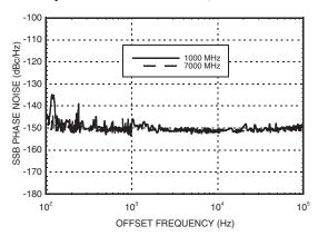
$<sup>\</sup>label{eq:continuous} \textbf{[1] Phase Noise Floor vs Offset Frequency over temperature}$
