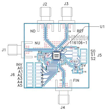
The circuit board used in the application should use RF circuit design techniques. Signal lines should have 50 Ohm impedance while the package backside ground paddle should be connected directly to the ground plane similar to that shown. A sufficient number of via holes should be used to connect the top and bottom ground planes. The evaluation circuit board shown is available from Hittite upon request.
