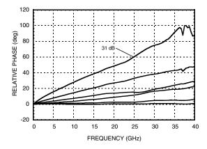
Step Attenuation vs. Attenuation State 18 - 33 GHz
