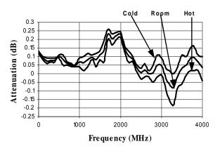
Typical Attenuation Deviation vs. Temperature for 4 dB Bit
