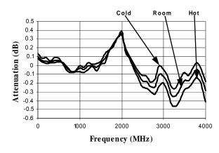
Typical Attenuation Deviation vs. Temperature for 16 dB Bit
