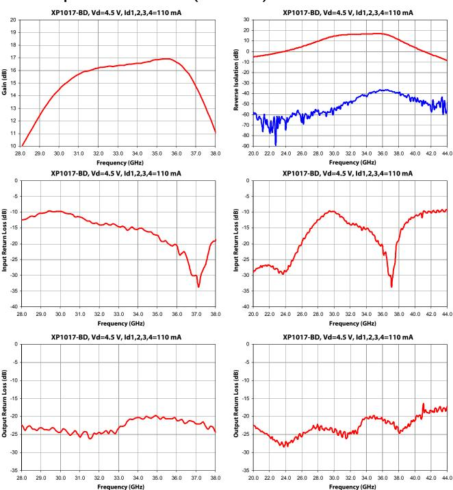
**Note** [1] **Measurements** – On-Wafer S-Parameters have been taken using reduced bias conditions as shown. Measurements are referenced 150 um in from RF In/Out pad edge. For optimum performance Mimix T-pad transition and tuned output matching network is recommended. For additional information see the Mimix "T-Pad Transition" application note. Contact technical sales for output matching network information.
