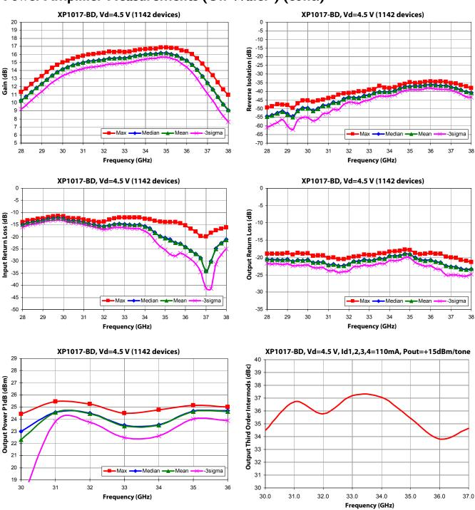
**Note [1] Measurements** – On-Wafer Output Power data has been taken using bias conditions as shown. Measurements are referenced 150 um in from RF In/Out pad edge. For optimum performance Mimix T-pad transition and tuned output matching network is recommended. For additional information see the Mimix "T-Pad Transition" application note. Contact technical sales for output matching network information.
