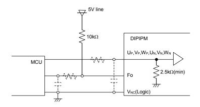
Note) RC coupling at each input (parts shown dotted) may change depending on the PWM control scheme used in the application and the wiring impedance of the application's printed circuit board. The DIPIPM input signal section integrates a  $2.5k\Omega(min)$  pull-down resistor. Therefore, when using a external filtering resistor, care must be taken to satisfy the turn-on threshold voltage requirement.
