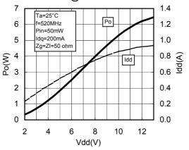
RoHS Compliance, Silicon MOSFET Power Transistor 175MHz, 520MHz, 2W
