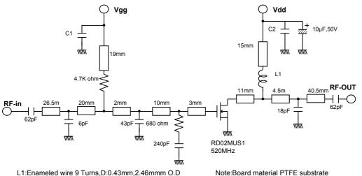
L1:Enameled wire 9 Turns,D:0.43mm,2.46mmm O. C1,C2:1000pF,0.0022µF in parallel Note:Board material PTFE substrate Micro strip line width=2.2mm/50 ohm,er:2.7,t=0.8mm
