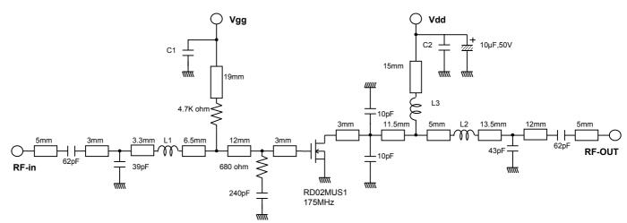
L1:Enameled wire 5 Turns,D:0.43mm,2.46mmm O.D L2:Enameled wire 3 Turns,D:0.43mm,2.46mmm O.D L3:Enameled wire 9 Turns,D:0.43mm,2.46mmm O.D C1,C2:1000pF,0.0022µF in parallel Note:Board material PTFE substrate Micro strip line width=2.2mm/50 ohm,er:2.7,t=0.8mm
