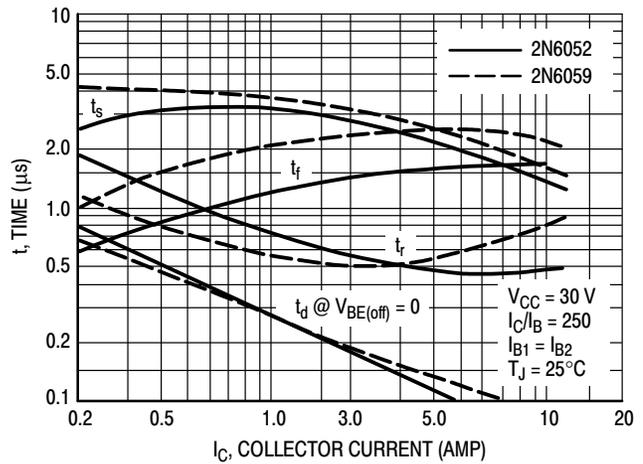
Figure 3. Switching Times
