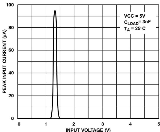
Figure 13. IN Pin Input Current vs. Input Voltage
