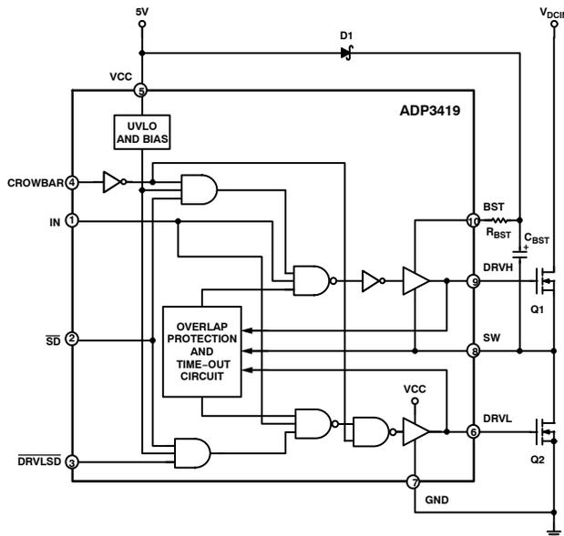
Figure 16. Detailed Block Diagram of the ADP3419
