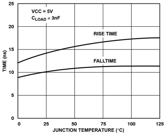
Figure 7. DRVH Rise and Fall Times vs. Temperature
