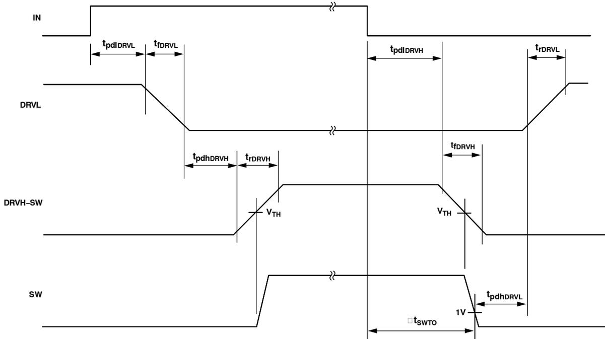
**Figure 4. Non-Overlap Timing Diagram**
