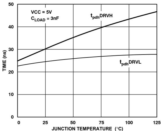
Figure 11. DRVH and DRVL  $t_{pdh}$  vs. Temperature
