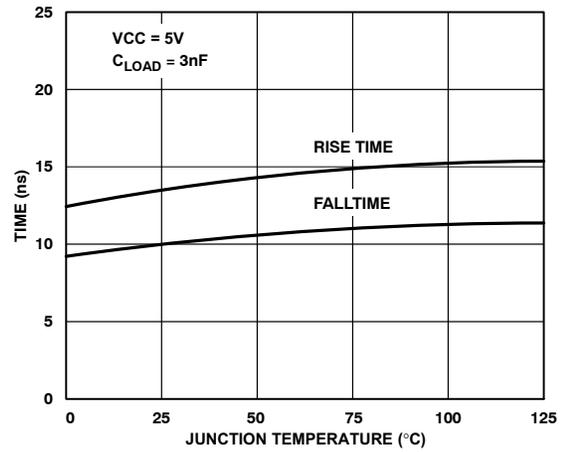
Figure 8. DRVL Rise and Fall Times vs. Temperature
