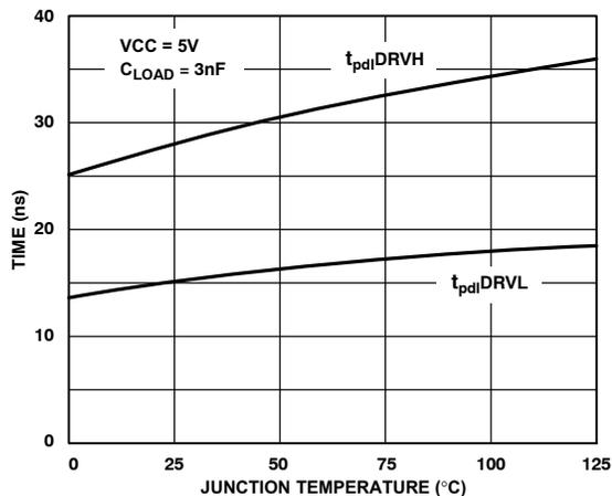
Figure 12. DRVH and DRVL  $t_{pdl}$  vs. Temperature
