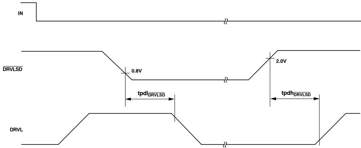
**Figure 3. Output Disable Timing Diagram**
