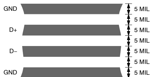
Figure 22. Typical Arrangement of Signal Tracks
