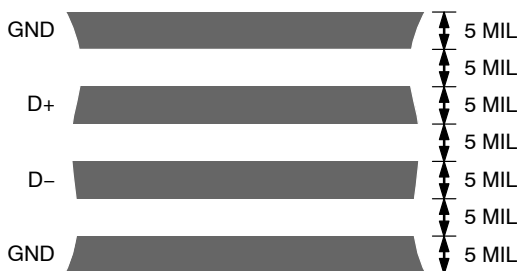
Figure 21. Typical Arrangement of Signal Tracks
