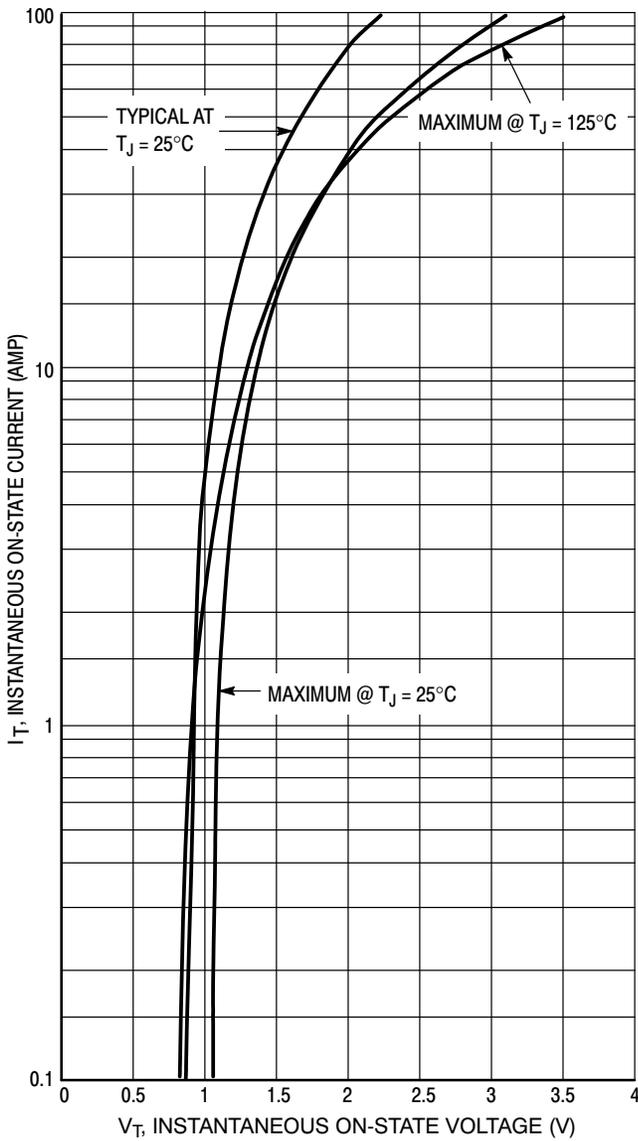
Figure 3. On-State Characteristics
