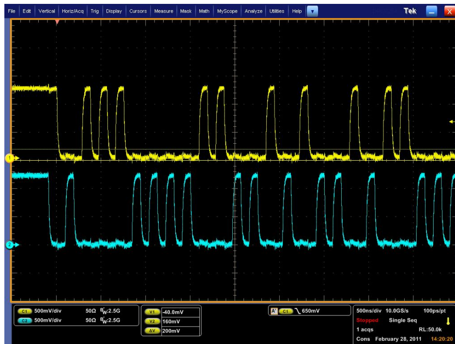
Figure 8. EMI4162MU MIPI D-PHY LP Mode Measured Results
