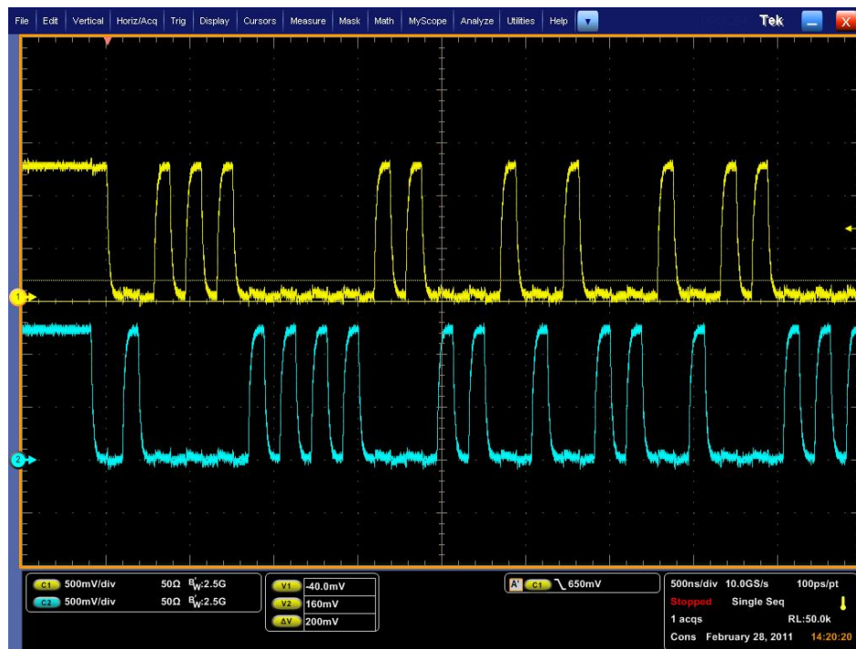
Figure 5. EMI4172 MIPI D-PHY LP Mode Measured Results
