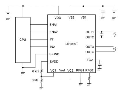
Channel 1 operates in constant voltage control mode: OUT outputs  $V_{DD} \times 3K/(3K + 6K) \times 1.95$ Channel 2 operates in constant current control mode: The RFG voltage is controlled so that Vref/4.5 = 0.2 V. \*: FC1 is left open.
