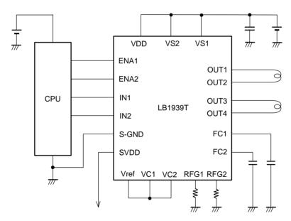
Constant current control mode: The RFG voltage is controlled so that Vref/4.5 = 0.2 V.
