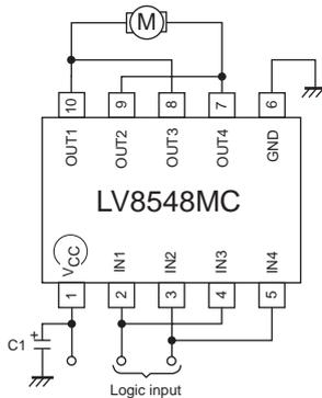
\* Bypass capacitor (C1) connected between  $V_{CC}$ -GND of all examples of applied circuit recommends the electric field capacitor of  $0.1\mu\text{A}$  to  $10\mu\text{A}$ .
