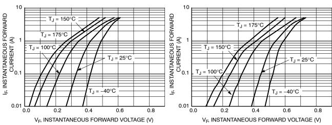
Figure 1. Typical Forward Voltage
