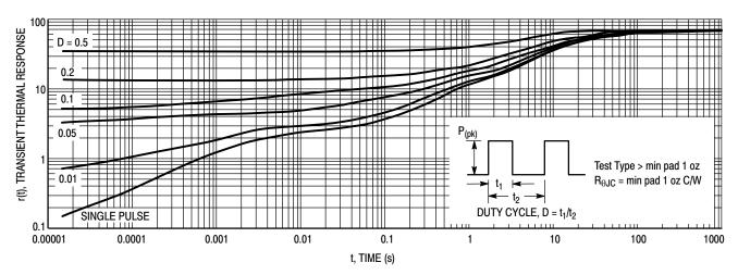
Figure 8. Thermal Response, Junction-to-Ambient, SMC Package
