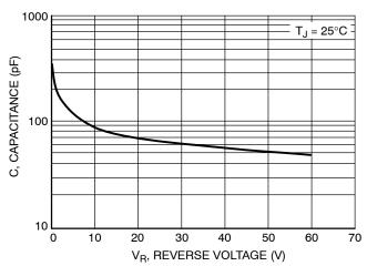
Figure 7. Typical Capacitance
