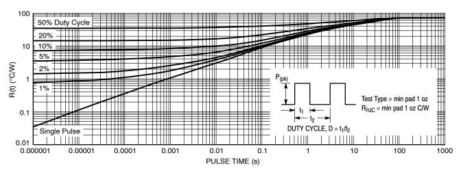
Figure 9. Typical Thermal Response, Junction-to-Ambient, SMB Package
