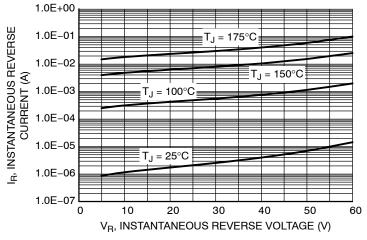
Figure 3. Typical Reverse Current
