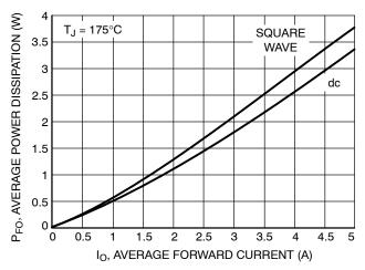
Figure 6. Forward Power Dissipation
