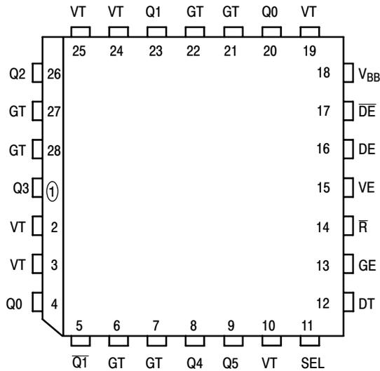
**Figure 1. Pinout: PLCC-28**
