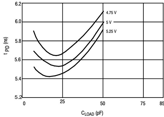
Figure 9.  $t_{PD}$  versus Load Typical at  $T_A = 25^\circ\text{C}$
