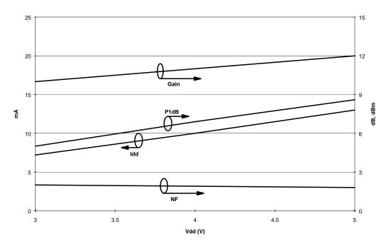
Typical Characteristics -  $V_{DD}$  = 5.0 V
