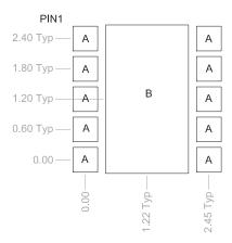
Figure 2. PCB Solder Mask Pattern (Top View)
