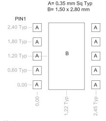
Figure 1. PCB Metal Land Pattern (Top View)
