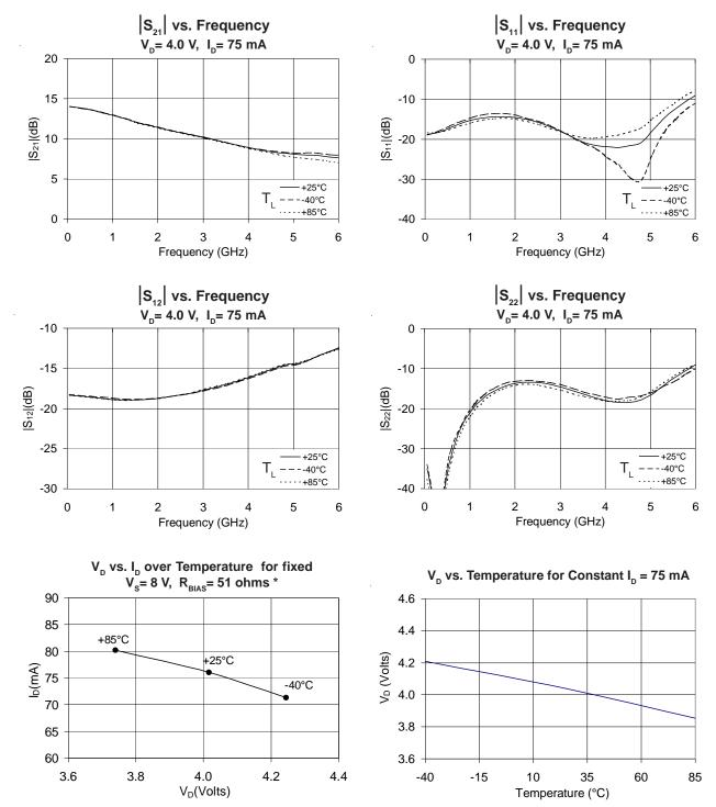
$<sup>^{\</sup>star}$  Note: In the applications circuit on page 4, R $_{\scriptsize BIAS}$  compensates for voltage and current variation over temperature.
