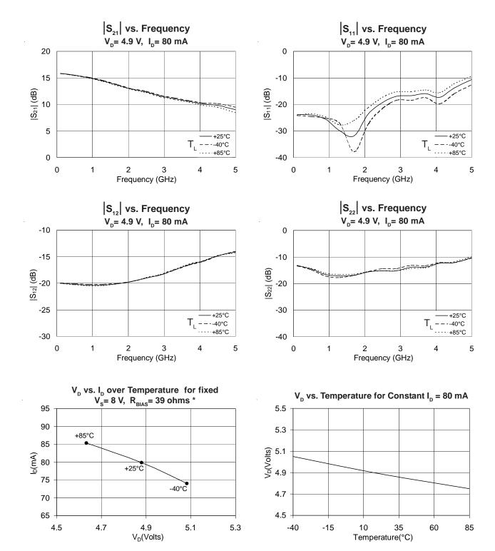
$<sup>^{\</sup>star}$  Note: In the applications circuit on page 4,  $R_{\scriptscriptstyle BIAS}$  compensates for voltage and current variation over temperature.
