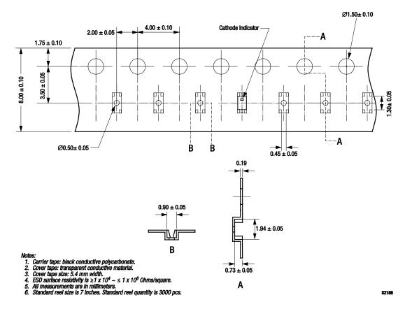
Figure 5. SC-79 Tape and Reel Dimensions
