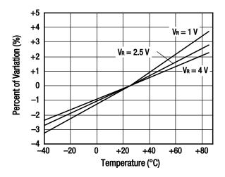
Figure 2. Relative Capacitance Change vs Temperature
