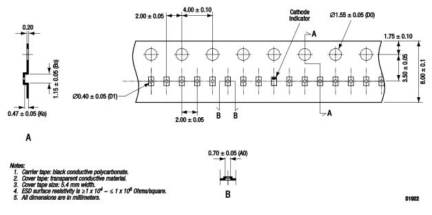
Figure 7. SOD-882 Tape and Reel Dimensions
