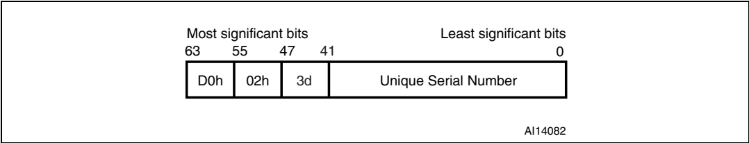
Figure 50. 64-bit unique identifier of the SRIX4K
